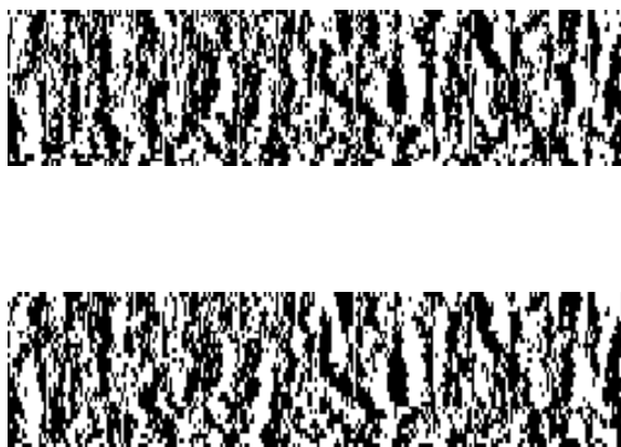
Figure 8: Two similar iris codes obtained for similar iris images ([15], 0001-L-0001.j2c, 0001-L-0003.j2c) using Gabor Analytic Iris Texture Binary Encoder
